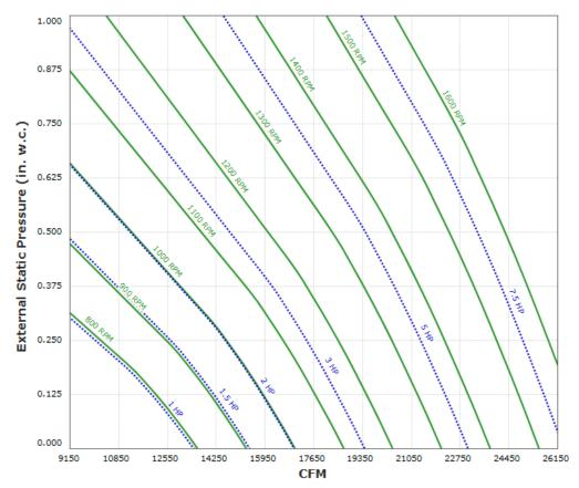
$\label{eq:max-size-able-RPM} \mbox{Max Sizeable RPM = 1600 RPM. Curve shown extended beyond this point for reference only.}$
